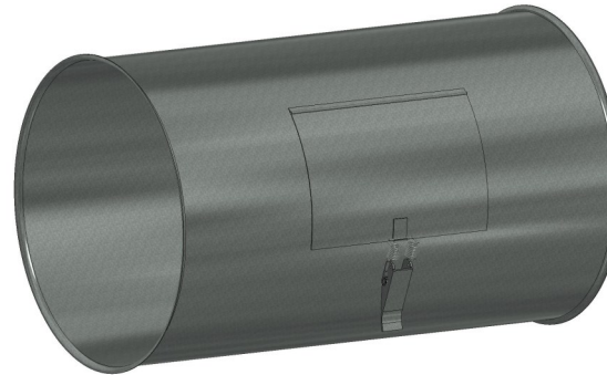
HINGED ACCESS DOOR ON 0.5M STRAIGHT DUCTING
